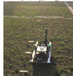
Figure 5. Robot "Ugo 1st" on landmine testfield at JRC - Ispra. The wooden arrows placed on the soil indicates the targets positions.
