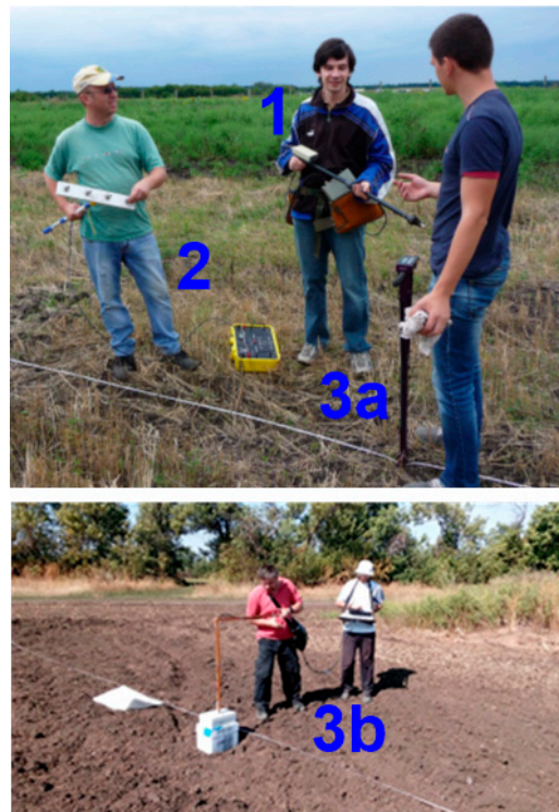
Figure 3. Photographs of field equipment. (1) Bartington MS2 magnetic susceptibility meter with MS2F probe, (2) L&R Instruments MiniRes with 4-electrode probe. (3a) Spectrum Technologies Field Scout 300 TDR. (3b) Purpose-built 1-Tx, 2-Rx impulse GPR.
