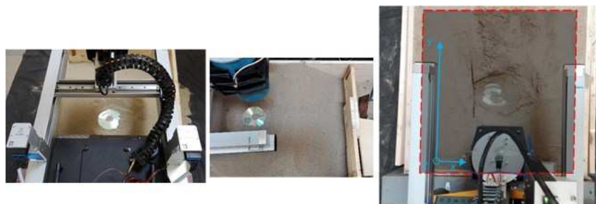
Figure 6: Pictures of the scanned area and the experimental setup with a CD in shallow sand.
