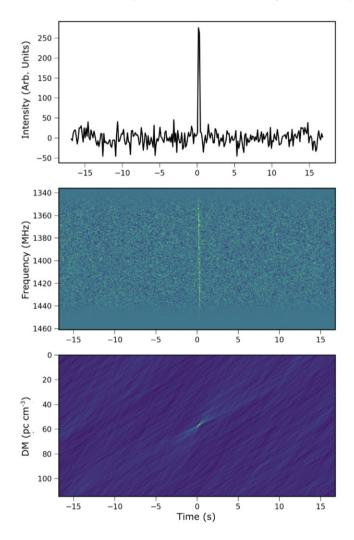
**Figure 3.** A sample pulse from the Crab Pulsar. The top panel shows dedispersed intensity versus time, the middle panel shows intensity versus dedispersed frequency and time, and the bottom panel shows DM versus time. This particular event has a DM of 57.17 cm<sup>-3</sup> pc and a S/N of 25.
