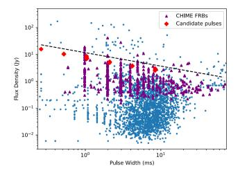
**Figure 5.** Flux density versus pulse width for known FRBs and our candidates. Known FRBs are in blue (Xu et al. 2023), the black dashed line shows the limit corresponding to S/N of 10 which extends over the range of pulse widths searched. The quantization seen for some pulse widths is due to the limited measurement precision of those entries in the database.
