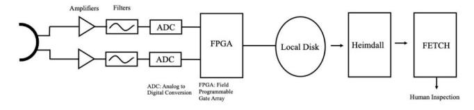
Figure 2. Schematic of the data acquisition and analysis pipeline, from the receiver to the final data outputs.
