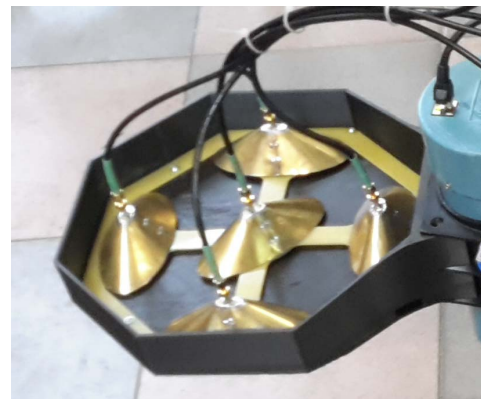
Fig. 4. 1Tx+4Rx antenna system for the impulse GPR is shown in the octagonal 3-D printed case.
