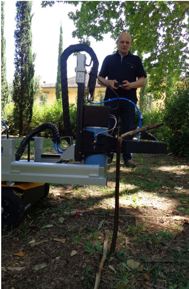
Fig. 6. Picture of the robot scanning a lane with width (30 cm) on a natural ground. Three buried targets (PMN-1, PMN-4 plastic-cased landmines and a metal tobacco tin) at depth about 5 cm and relative distance about 50 cm.
